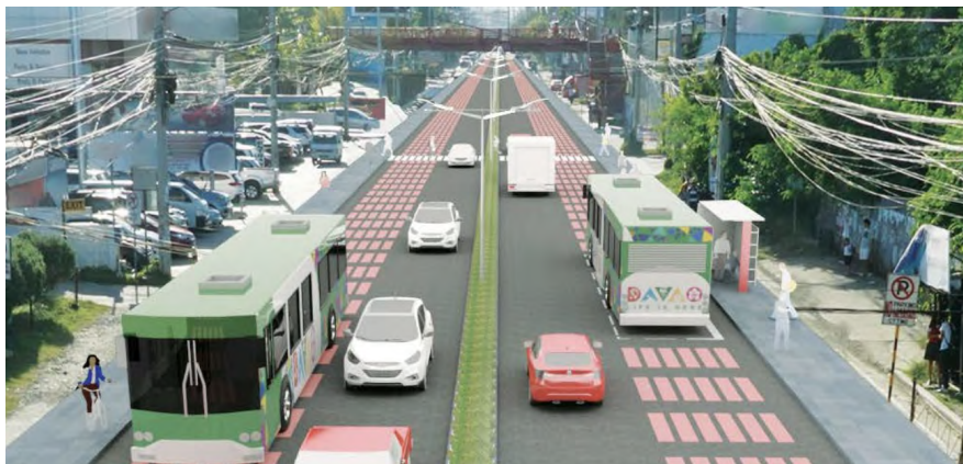
A COMPUTER-GENERATED VISUAL REPRESENTATION OF THE DAVAO HIGH PRIORITY BUS SYSTEM, INCLUDING THE BUSES, WAITING SHED, AND ROAD DESIGN.
